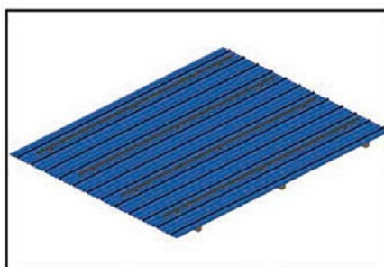
Step 2: Fix solar rail on L foot and lock by T modules set.
