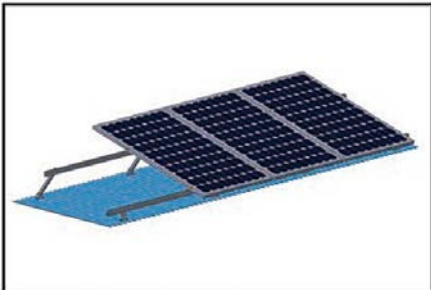
Step 3: Put solar panel on rail and fix with solar clamp until finished.
