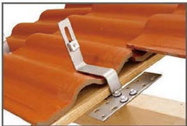
Step 1: Remove tile and fix tile hook on beam by M6.3 x 80mm wood screw.
