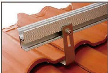
Step 2: Fix solar rail on tile hook and lock tightly by M8x2Smm T module set.
